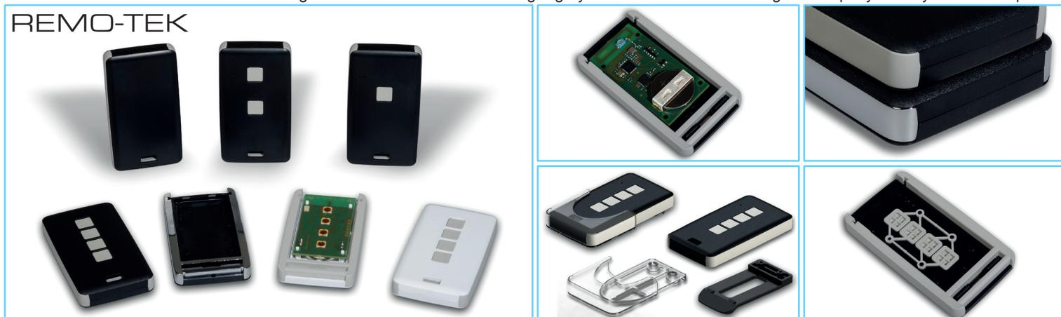
Remote control case featuring rounded edges available both as compact unit (13120) and with push button combination from one to four (13121, 13122, 13124). Internal pillars for PCB fixing. Two colour versions: white/light gray and black/light gray. Protection bumper in plastic or polished chromed metal. LED hole on the cover. One screw closing. Suitable to accept button cells, accessorizable with battery holder AB2032, wall mounting holder MT8 and belt clip CLP.
